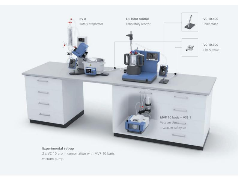
The application example shows two VC 10 pro vacuum controllers connected to one vacuum source. A VC 10.300 check valve has been installed between the MVP 10 basic vacuum pump and each of the vacuum controllers. Depending on the power of the vacuum source, the number of supplied controllers can be multiplied.
